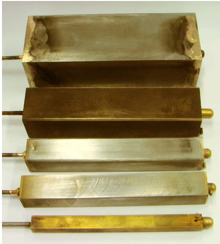
FIG. 6. (Color online) A photograph of the (brass or stainless steel) rods of square cross section that we have studied. They have cross sections of 5 \times 5 , 3 \times 3 , 2 \times 2 (with rounded corners), 2 \times 2 , and 1 \times 1 \text{cm}^2 .
