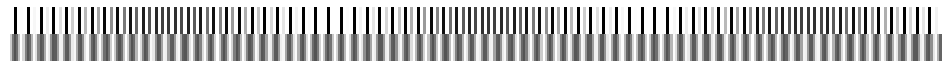
Fig. 18. The Kell artifact. The upper stripe represents discrete display showing a pattern 1 + \cos(\pi kx) for k = 0.98 , where x \in \mathbb{N} is the number of a pixel in a row. To emphasize the effect by reducing attenuation of the U_K(f) distortion, the pixels are interleaved with a white space of twice their width (this corresponds to real LCD, displaying red color with blue and green subpixels turned off). Three ‘beats’ of the artifact pattern can be seen there. The period of the error term’s factor \cos(\pi(1-k)x) is \frac{2}{1-k} = 2/0.02 = 100 . There are two visible beats per period due to the factor \cos(\pi x) = (-1)^x . As the display is 146 pixels wide, it gives 3 beats. The stripe below contains thrice as many pixels placed next to each other without gaps, showing the same signal. The Kell artifact is hardly visible there. The upper stripe would look similarly had it been filtered by proper interpolating filter. Due to nonlinear dependence of blackness (which is hard to be completely compensated by a gamma correction, owing to paper and ink aging) there is also an aliasing artifact present. The aliased third harmonic has a period of 2.13 pixels (of the upper display), while for the second one it is 50 pixels, the same as the beating period. However, the aliasing leads to purely sine waves without the (-1)^x modulation factor that is clearly visible in the figure, which shows that we really see the Kell effect. Even higher harmonics are of negligible amplitude in comparison to \alpha \approx 1 of the error term.
