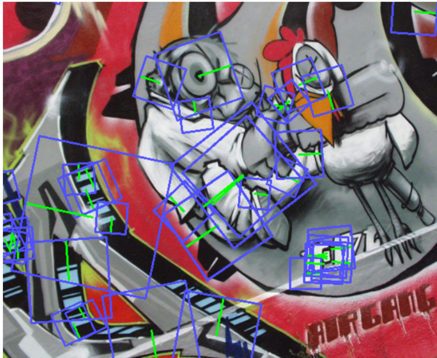
Figure 3.4: Description windows with size 20 times of the detected scale. The dominant direction is shown by a green line.
