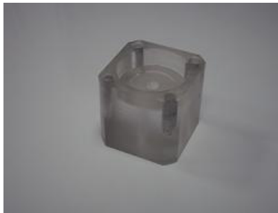
Figure A.1: Collimator for scintillators and diode testing with RS.
