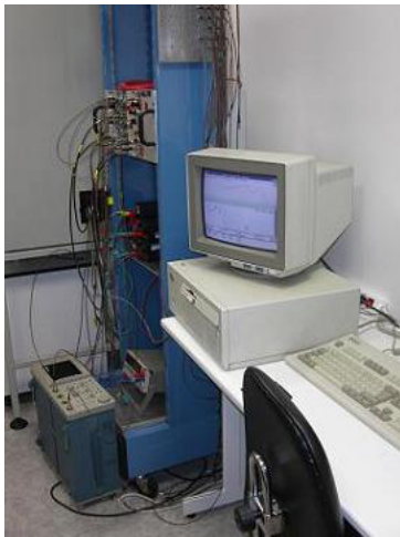
Figure A.7: The multichannel readout analyzer and oscilloscope.
