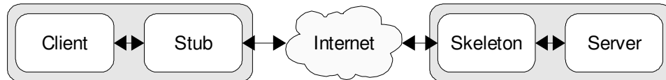
Figure 2.1: A typical implementation of Java RMI. Stub and Skeleton are special intermediate objects.
