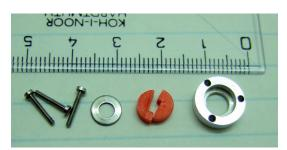
(ii) A metal-plastic clamp for a single probe. The eligibility of such a construction is in repeatability in placement of numerous probes (but those differing in length only, with a specified cross-section).
