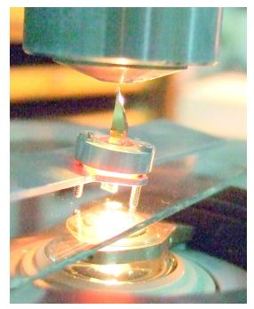
(i) The probes were hold in a metal-plastic clamp for a single probe. Here, the clamp with a probe is photographed being above a microscope light and under a microscope ocular. The parts of the clamp are in (ii)
