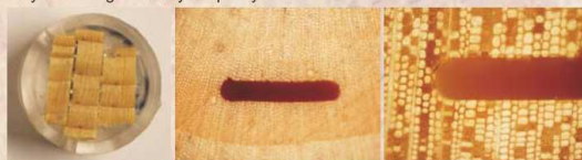
Sample mount and laser ablation pits in tree rings (track length is 600 microns).
