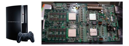
Figure 2.2: Images of Cell/B.E. based machines. Sony's Play Station 3, on the left (image taken from www.boygeniusreport.com), IBM Cell Blade board, on the right (image taken from www.ps3tester.com)
