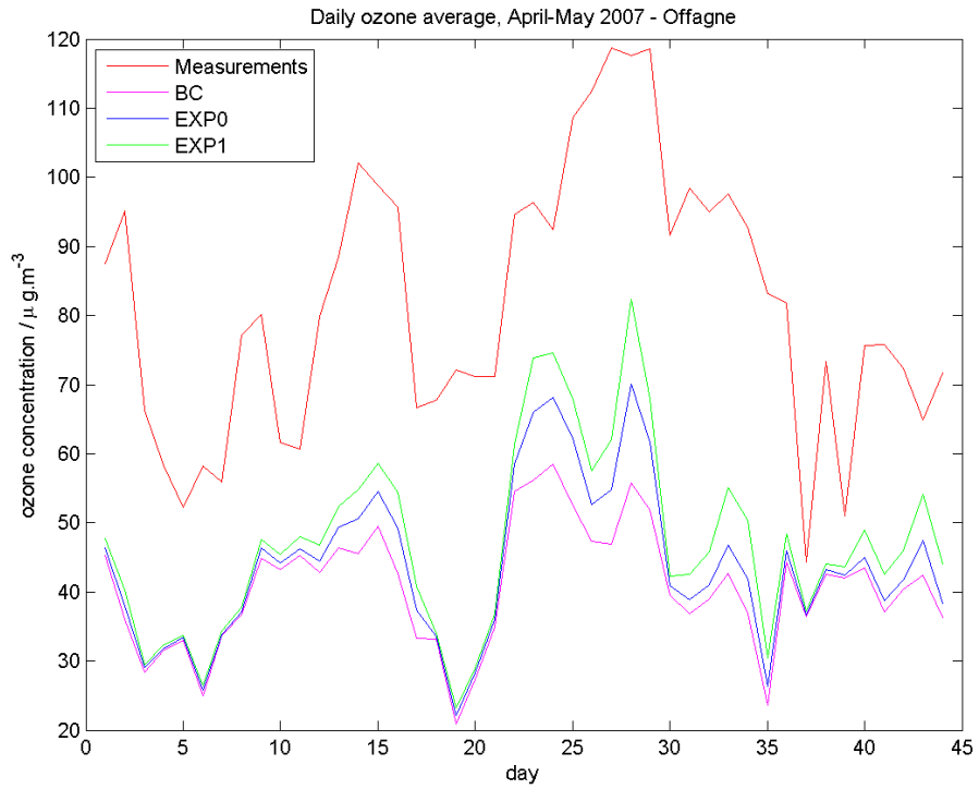
Figure 7.20: Daily mean ozone concentration ( \mu\text{g}\cdot\text{m}^{-3} ) measured at Offagne station compared to model simulations.
