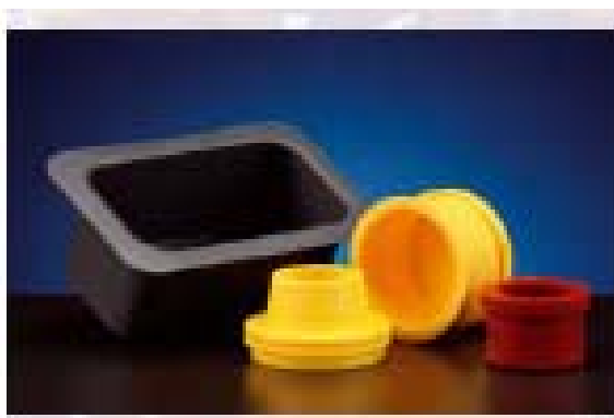
FIG. 10 VARIOUS TYPES OF MOUNDING CUPS (yellow cups were used for the needs of this study)
