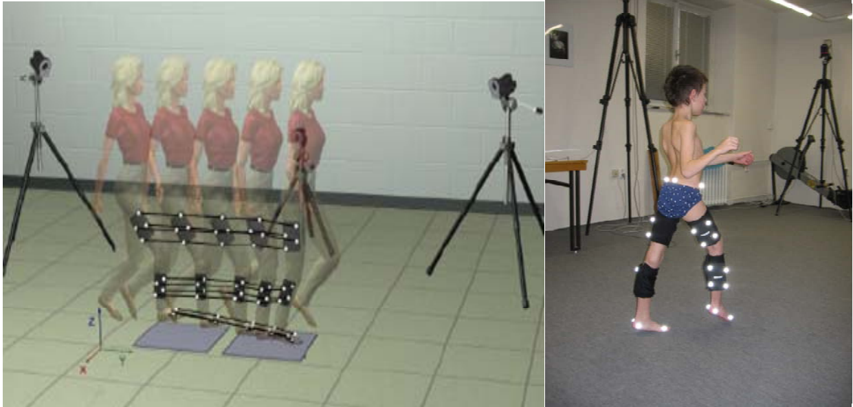
Figure 8. A drawing and photograph of a child walking through the calibrated volume during the gait analysis. Three dimensional marker tracking is graphically demonstrated.
