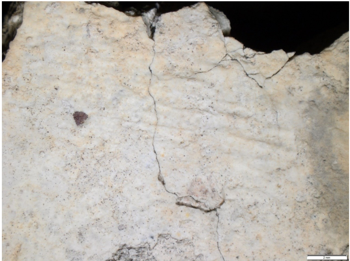
Figure 43) Microphotograph of sample NPT 11 with evidence of brush or tool marks on the finishing surface. The finishing layer is completely white, with no traces of pigments. The slight yellow to pink spots are caused by the depositional context of the sample, which is characterized by a soil rich in iron content, similar to terra rossa. Furthermore, certain types of microorganisms' decomposition can cause this type of red stains on the surface.
