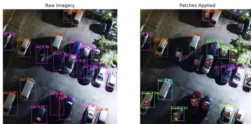
Figure 3. Adversarial patches digitally added to the image on the right caused invisibility or misclassification of vehicles. Proposed by Van Etten in “The Weaknesses of Adversarial Camouflage in Overhead Imagery.” Proceedings - Applied Imagery Pattern Recognition Workshop . © 2022, IEEE
