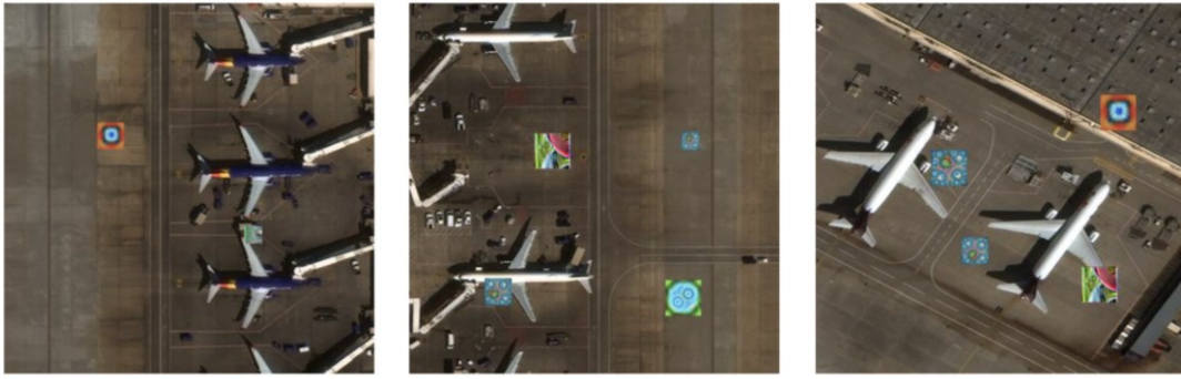
Figure 4. Legacy adversarial patches applied on the aircraft stand by Van Etten in “The Weaknesses of Adversarial Camouflage in Overhead Imagery.” Proceedings - Applied Imagery Pattern Recognition Workshop . © 2022, IEEE
