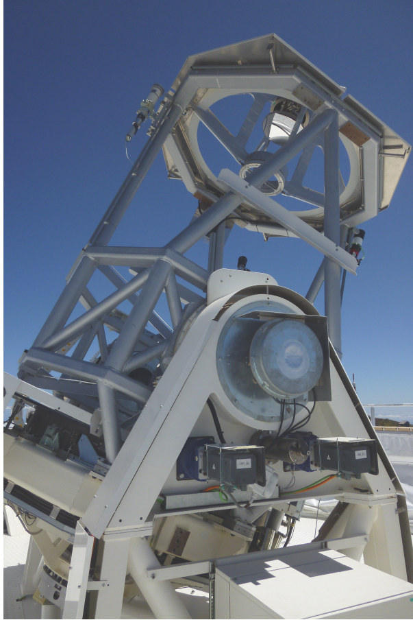
Figure 3.2 GREGOR secondary mirror and the mechanical structure at the dome.
