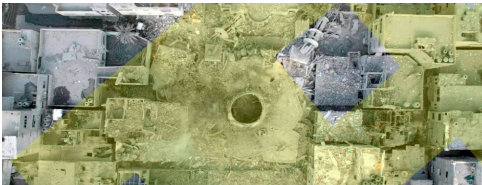
Figure 12: Georeferenced drone footage of Ahmed Yassin mosque post-airstrike (October 9) with 20-meter threshold change mask overlay
