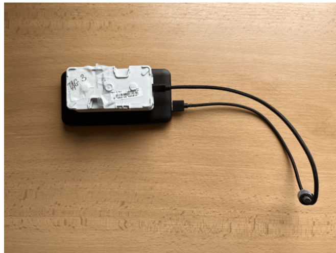
Figure 3.9 An example of a protective box that is used to protect ESP32 UWB boards.
