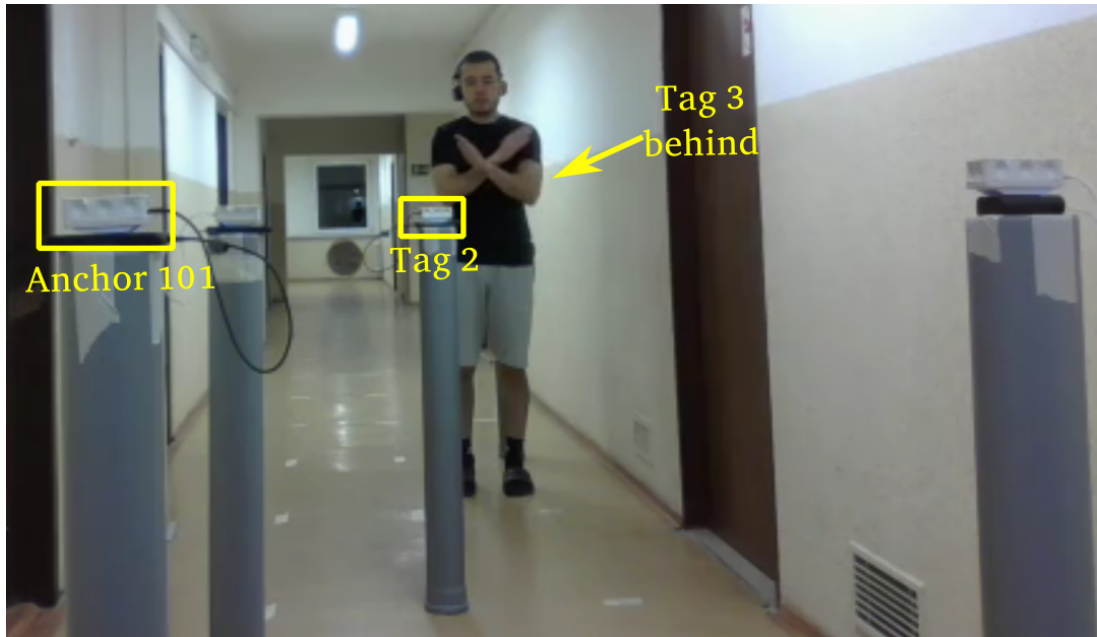
Figure 3.25 A person blocks the communication between the anchor and tag (behind person).
