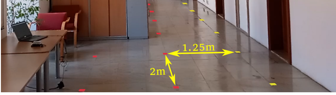
Figure 3.10 An example of the reference system used during our experiments. The stickers are placed in three rows, maintaining an interval of 1.25 meters between each row and a 2 meter space between the stickers within a row.
