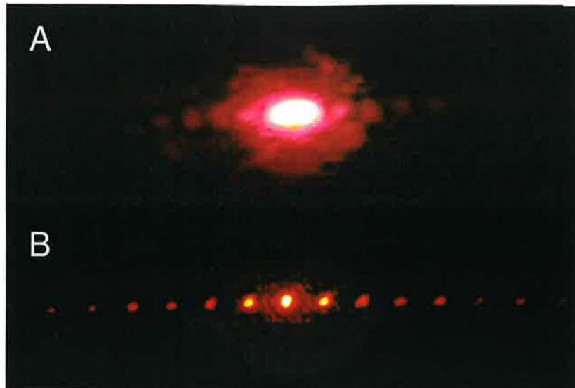
Figure 33: Pattern of a laser beam diffracted on a grating burned in the sample. (A) An excitation with ns laser pulses, (B) excitation with fs laser pulses.
