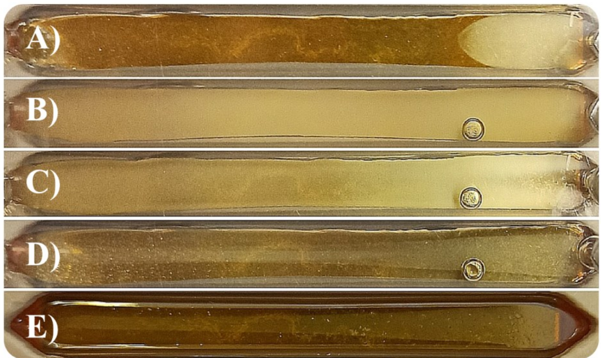
Figure 18: With the medium flow rate 0.2 mL/min, it takes approximately 10 minutes for the bacterial suspension to fill the whole chamber (A and B). Introduction of fresh medium after the 4 hours of inoculation initiates washing off weakly attached cells (C), and 24 hours of growth a biofilm is observable through the lid (D) just as well as without the lid (E).
