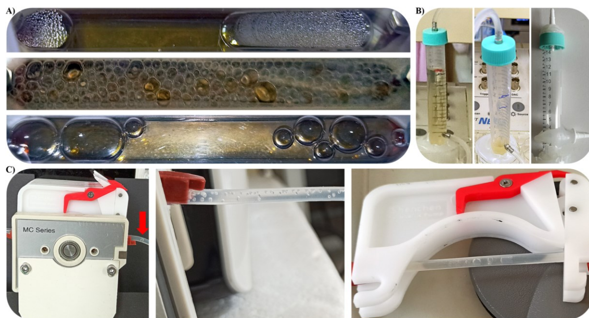
Figure 12: Polycarbonate lid enables observing air bubbles inside the flow cell by the naked eye
