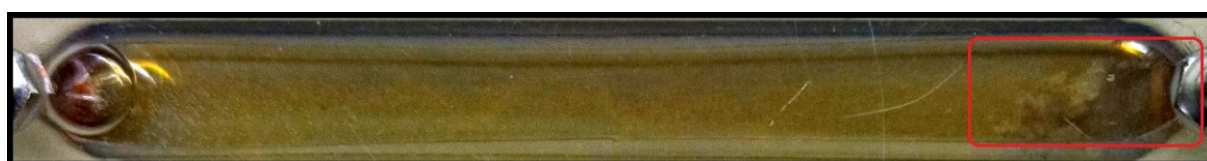
Figure 47: Flow cell biofilm damaged during the exchange of supply bottles (red rectangle).
