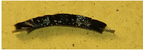
(a) Side view of TPU + Nitinol composite after TMA testing
