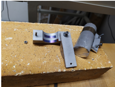
(a) Sample in bending mould after annealing
