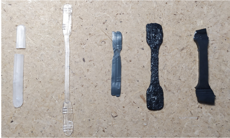
Figure 5.10 3D printed samples of polymers after testing, starting from left: PLLA annealed, PLLA unannealed, HD PLA, CoPa and TPU60&PCL40
