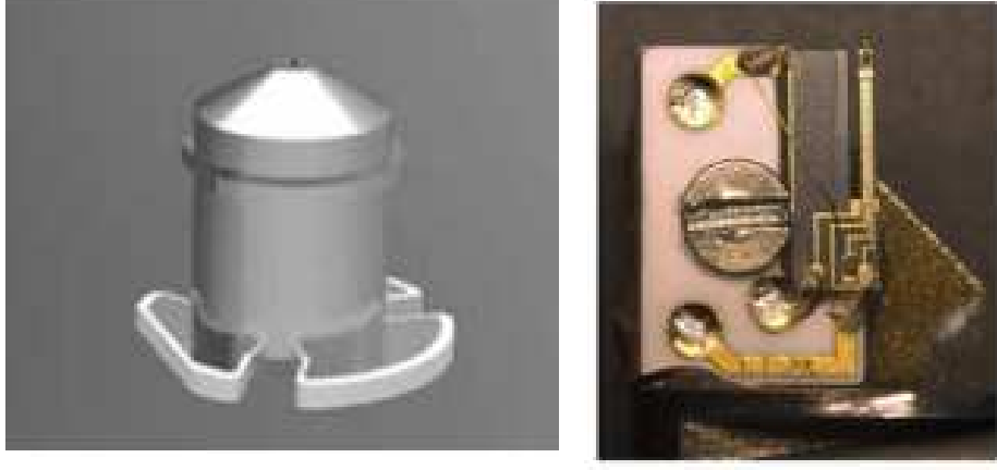
Figure 1.8: A Kolibri (left) and qPlus sensor (right)
