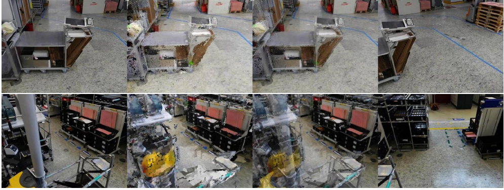
Figure 3.14: The first column shows the query photo, the second render of the best candidate position, the third a blend of the two preceding columns and the last column shows the database photo obtained from the image retrieval step. The upper row shows an error of 0.01 m and 0^\circ , the second an error of 0.18 m and 1^\circ . On the query image of the second row, there is also visible the relic of the reprojection from panorama photo to 2D photo on the tubes in the foreground.
