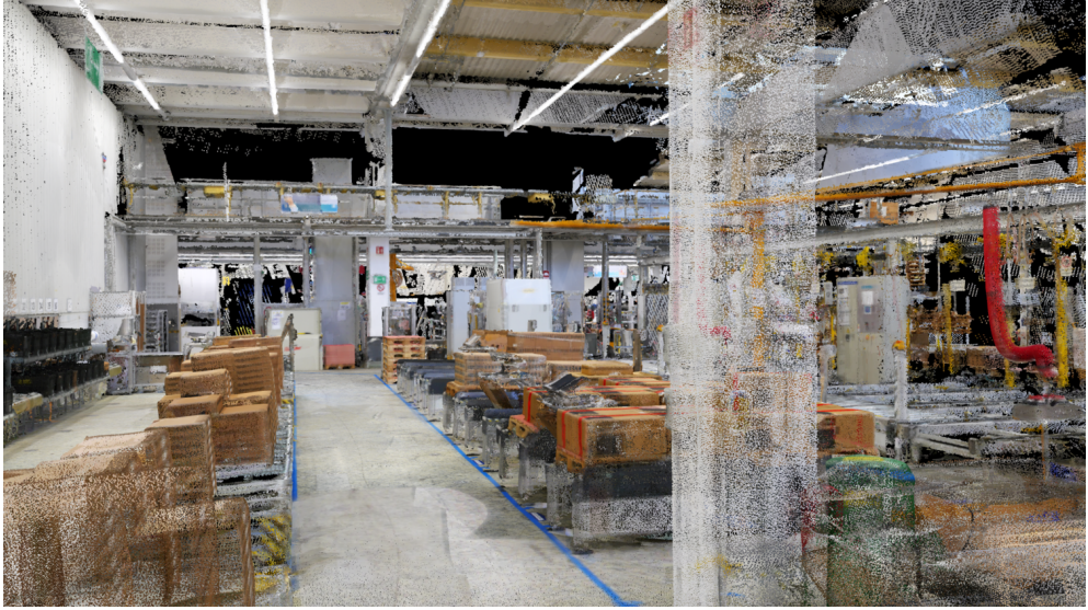
Figure 1: A render of one of the datasets’ point cloud. We can see an issue with using OpenGL’s point primitive. Closer surfaces (the column, for instance) to the camera are not continuous but have holes and points that should be occluded by closer surfaces being visible. Fixed screen space point primitive is thus not a reliable way of rendering a point cloud without per-render pre-computations to set the correct pixel primitive.
