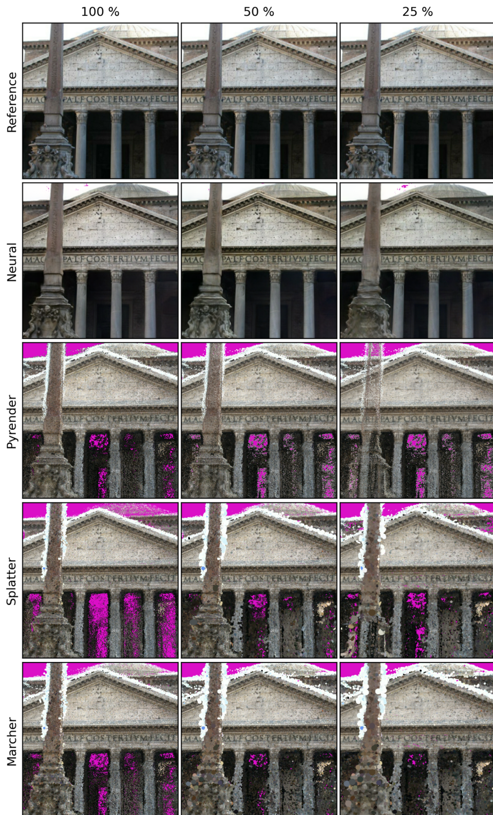
Figure 3.12: Visual comparison of various renderers and point cloud densities for Pantheon Collection. Contrastive background color is displayed, Open3D’s voxel downsampling is used for point cloud simplification.
