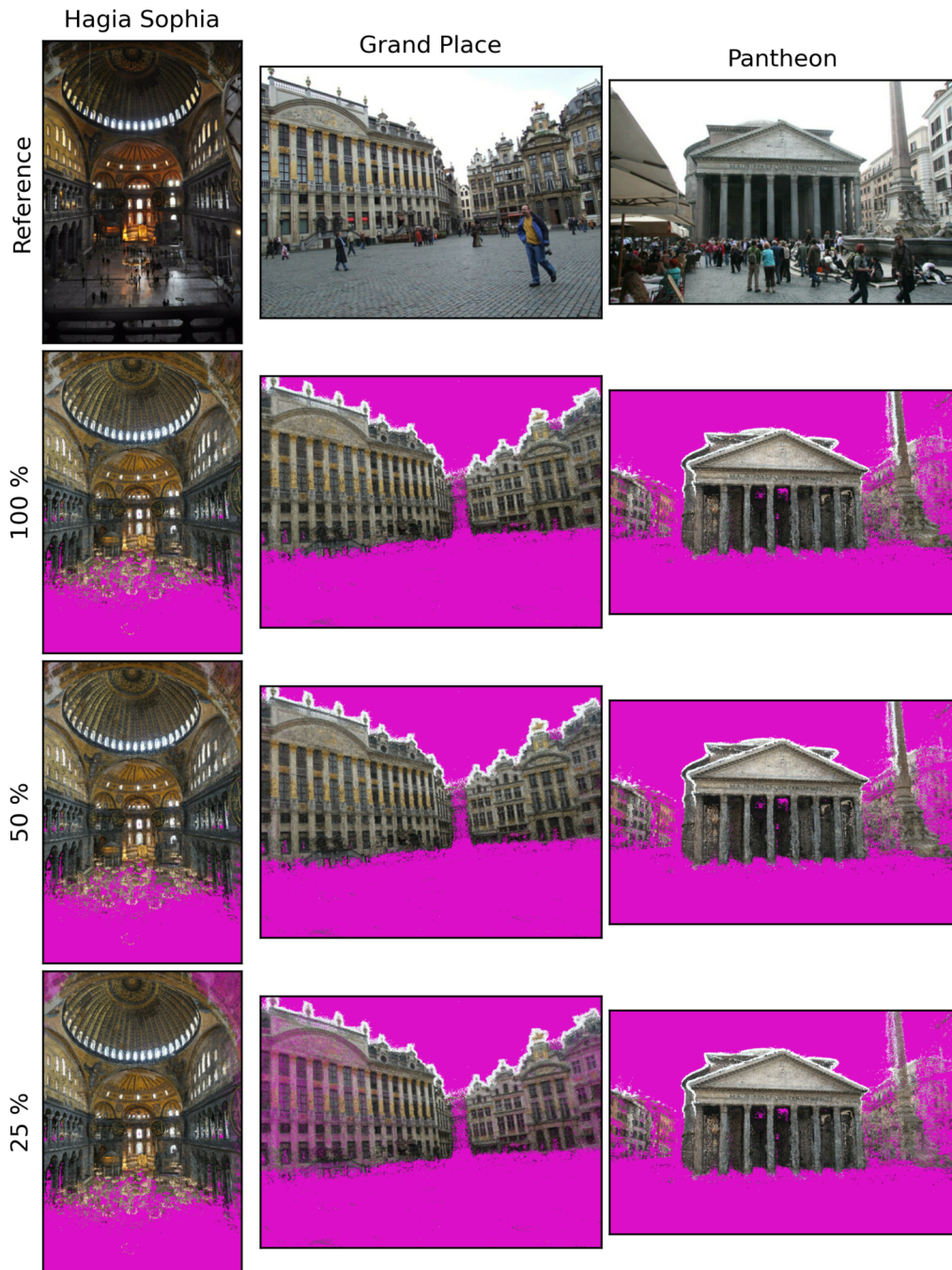
Figure 3.9: Visual comparison of point cloud density influence on rendering. The renders are produced by Pyrender ( GL_POINTS ) with contrastive background color to present the differences better. Point cloud simplification is done by Open3D’s voxel downsampling to preserve the original structure with fewer points. The downsampling method proceeds in two steps; firstly, points are bucketed into 3D volumes called voxels , each resulting in exactly one point of the simplified output by averaging all points inside the source voxel in the second step. Since Pyrender has a fixed point size in screen space, its disadvantage can be seen—closest portions of the scene look sparser than the farther portions.
