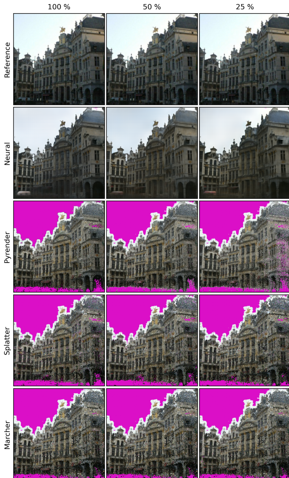
Figure 3.11: Visual comparison of various renderers and point cloud densities for Grand Place Brussels Collection. Contrastive background color is displayed, Open3D’s voxel downsampling is used for point cloud simplification.
