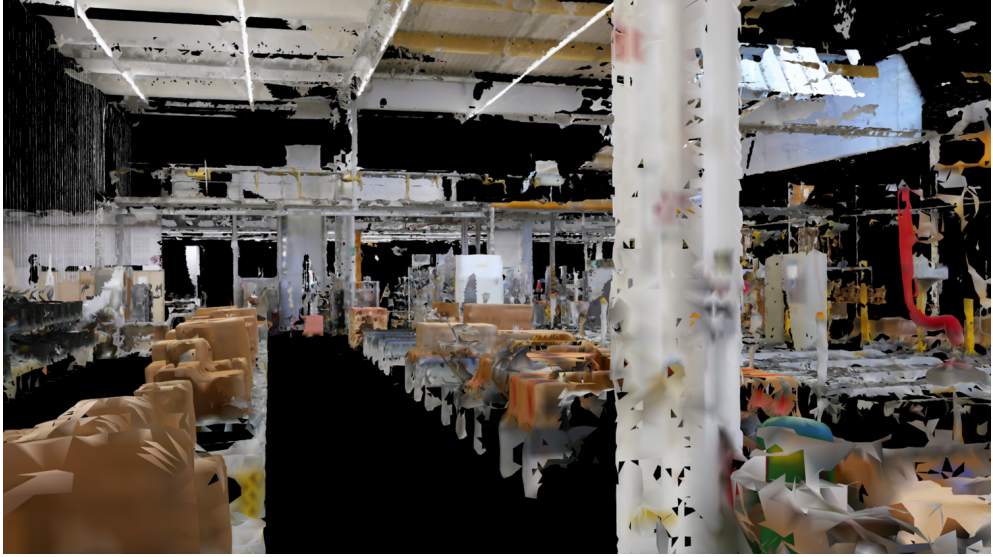
Figure 2.1: A render of one of the meshes created from the raw datasets’ point cloud, camera pose is the same as for Fig. 1. The mesh was created semi-manually, meaning that boxes, for instance, were meshed separately and then placed at the right place of the resulting mesh. We can see some disadvantages of using meshes in complex environments. Despite long processing time and laborious manual work, the result is not compelling compared to renders using point primitives.
