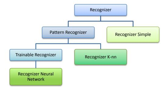
Figure 5.3: Recognizer class hierarchy
