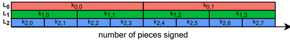
Figure 2.2 The expected key lifetime ratios on different layers with \text{KEY\_RATIOS} = [(4, 0), (2, 0), (1, 0)] . One can see that keys from L_0 sign two times less frequently than L_1 and four times less frequently than layer L_2 .
