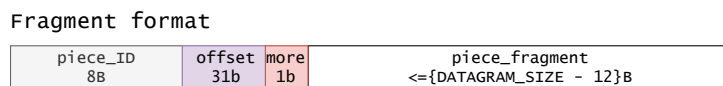
Figure 2.5 The format of a fragment that is then passed to the network interface for the transfer.
