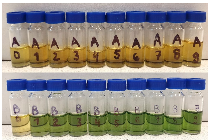
Figure 16: Samples of reaction mixtures: blank (up) and with Cu/Beta catalyst (bottom), centrifuged
