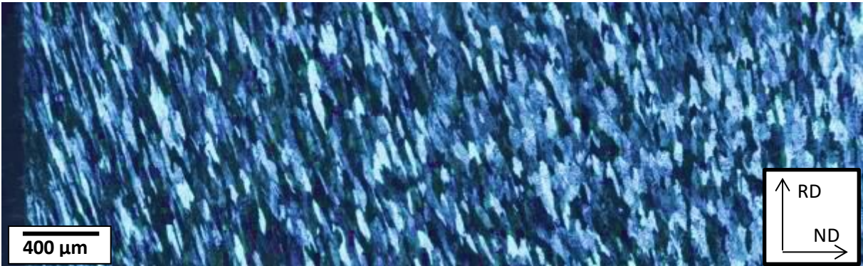
Figure 4.4: Grain structure of the cast strip cross section
