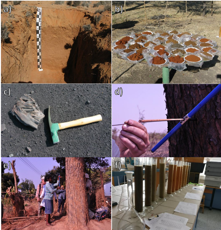
Figure 6 Overview of sampling and sample handling. a) Example of an open pit from which soil samples were gathered. b) Soil samples left in the sun for air-drying to constant weight. c) A slag found in an open-air slag dump with a geological hammer for scale. d), e) extraction of a tree ring core using a Haglof incremental borer collected at chest height. f) Granulometry determination using the sedimentation method.
