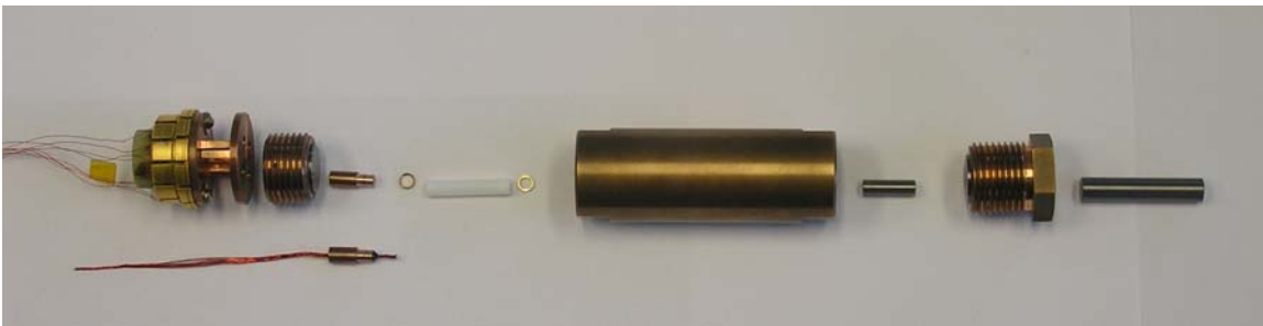
Fig. 4.1 The new pressure cell (from left to right): Puck for connection with PPMS, clamping bolt, plug, sealing rings and a Teflon capsule, body of the cell, piston, clamping bolt
