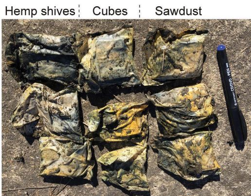
Fig. 1. Experimental double bags with NOM (hemp shives, wooden cubes, sawdust) after their incubation in the Mokrsko (M1) wetland. Note the characteristic yellow (AsS phases) and black (FeS phases) precipitates formed on the inner bag and on the surface of the NOM.
