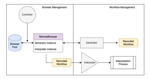
Figure 2.5: Server architecture diagram
