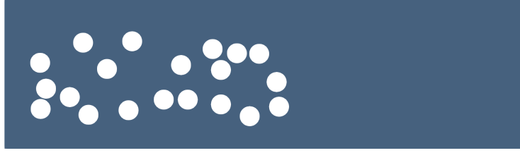
Figure 4.6: Initial random particle cluster used in the problem with linear initial velocity profile with 20 particles. The domain is more narrow than in the problem with stationary initial condition. In the problem with 40 particles, the initial cluster is wider. In the case of the particles in a grid, we used a 5 \times 4 and 10 \times 4 grid.
