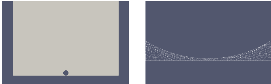
Figure 3.5: The solution with a no-slip boundary condition at time t = 5 \text{ s} . The circular particle completely stops around t = 2.25 \text{ s} and we see no significant particle movement after this time. The particle is divided from the boundary by two layers of elements.
