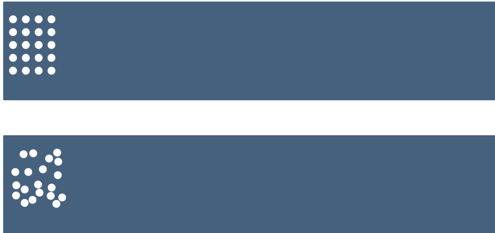
Figure 4.2: The fluid domain \Omega_0 with a particle cluster in a grid (top) and distributed randomly (bottom). To obtain a random distribution, we sample points uniformly in a chosen rectangle, if a choice of a point would cause an overlap, we sample again until there is no overlap. To keep the cluster consistent between different runs, a common initial seed is chosen to initialize the random number generator.
