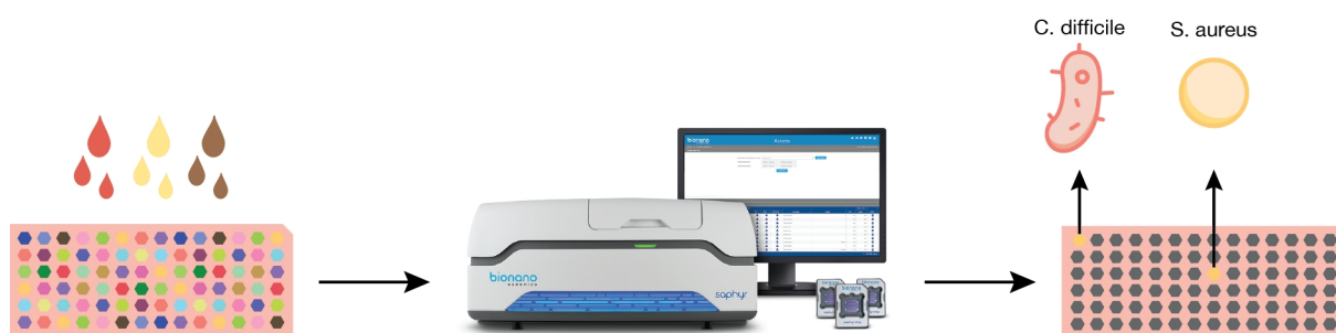
Figure 32. An overview of a possible high-throughput system that utilizes Supernova-based sensors. In this case, a chip containing a number of sensors specific for a variety of human pathogens is incubated with a sample from the patient. After the addition of CDP-Star, a reader determines which pathogen(s) are present based on which sensor(s) produce light. Based on the speed of the Supernova sensors specific for oligonucleotides, the whole process should not exceed 15 to 30 minutes.
