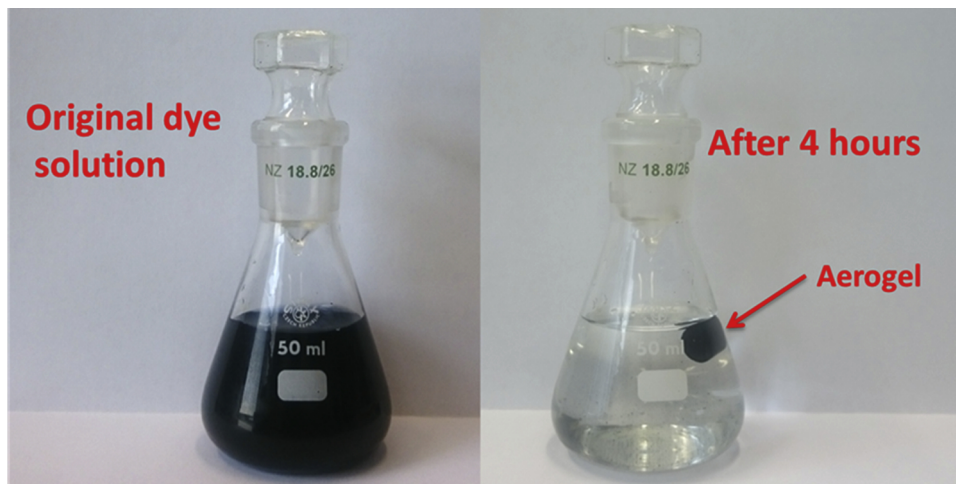
Fig. 5. The aqueous solution of Reactive Black 5 becomes colourless after immersion of a magnetic PANI/PVAL/2%F aerogel for 4 h.
