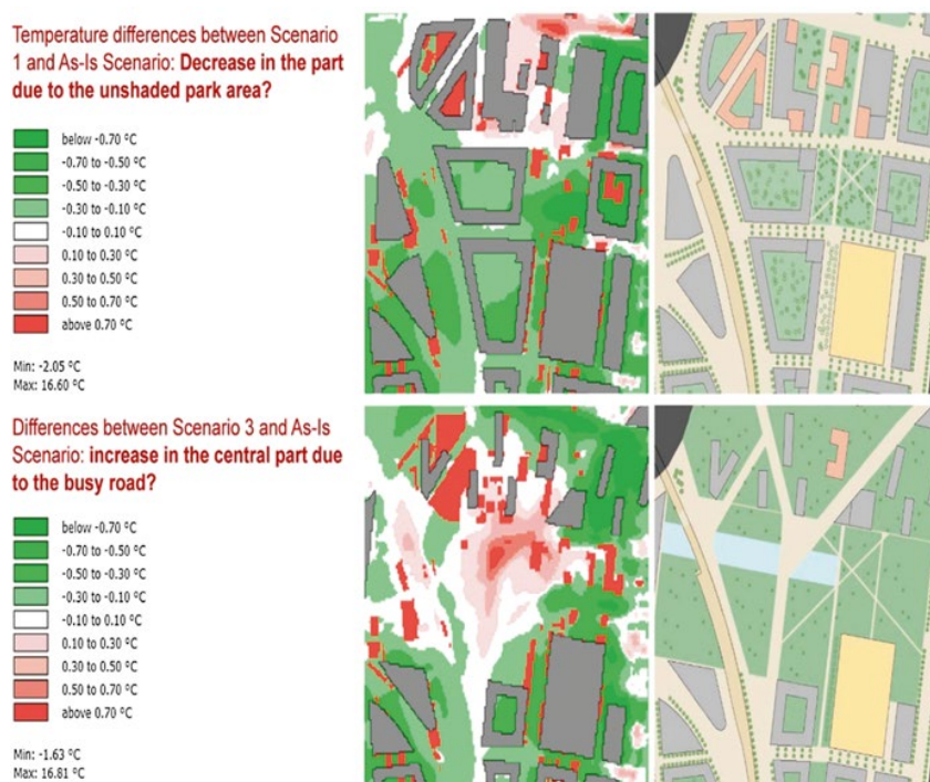
Fig. 14.30 The cooling effect of green roofs is negligible
