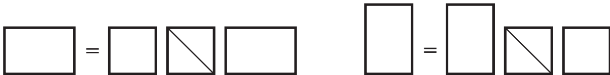
Figure 2.1: Singular Value Decomposition scheme. The figure shows dimensions of matrices in the equation (2.1). Left and right case correspond to n_A \leq n_B and n_A \geq n_B respectively. (from Schollwöck [2011])
