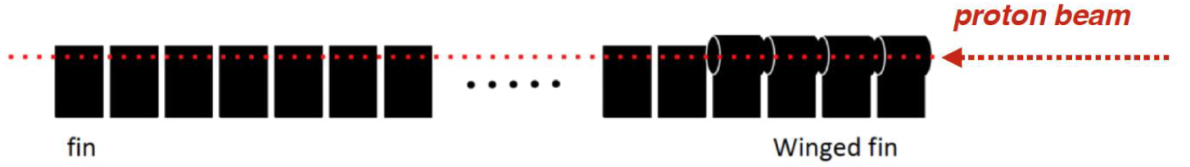
Figure 2.3: Schematic of the NuMI target graphite fins and four new winged fins to protect the beam components from any proton mis-steering, from Ref. [93].
