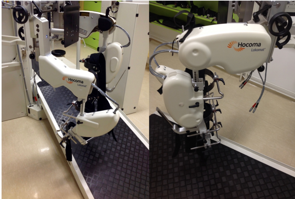
Figure 5: Lokomat Pro pediatric (left) and adult orthoses (right) (source: own).
