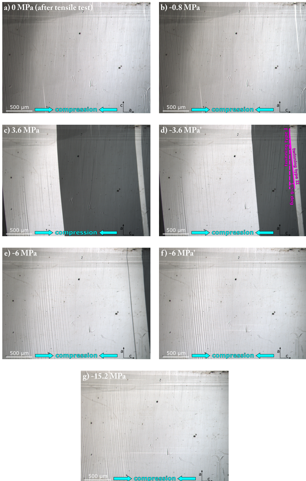
Figure 6.7: The micrographs of the C initial sample surface obtained from the optical microscopy during compression. The compression direction is indicated by the blue arrows. The black arrows indicate the presumed crystallographic axes of the initial state.
