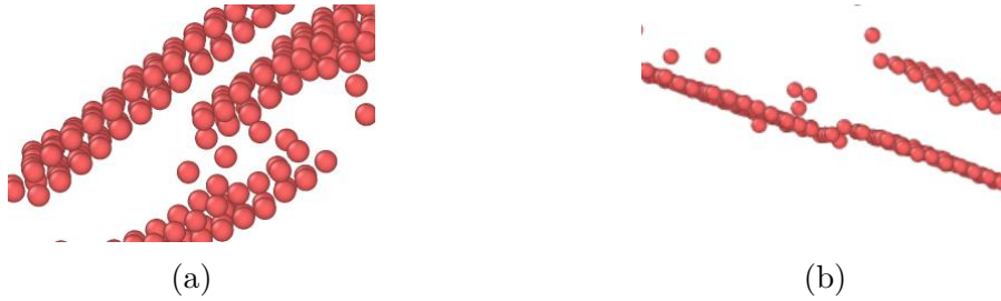
Figure 5.11: Comparison of HCP atom planes in a) Al-Si-Mg-Cu-Fe MEAM, b) Al MEAM.
