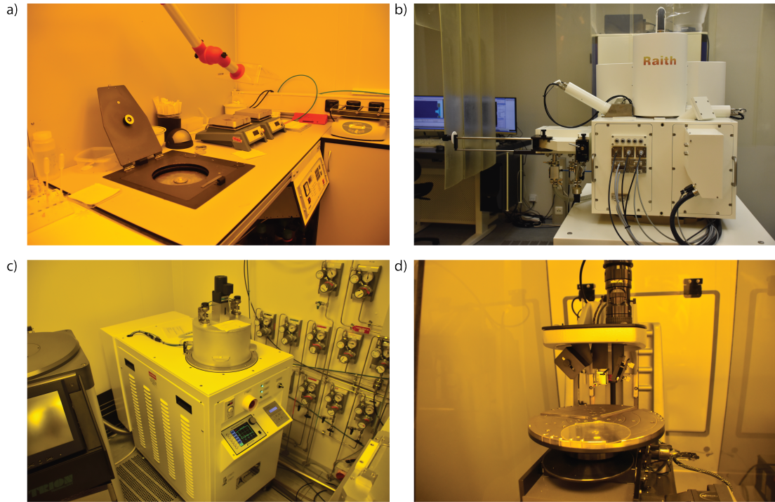
Figure 2.5: Different machines used in lithographic process. a) Spin-coating machine with hotplates behind it. b) Raith E-line electron beam lithography machine. c) Vapour deposition machine. d) Dektack surface profiler.
