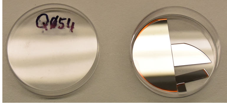
Figure 2.3: Example of CuMnAs thin film grown on GaP substrate wafer. This wafer is then cut into individual samples.
