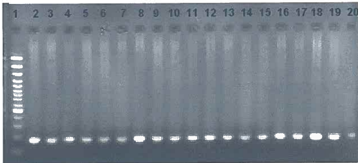
Fig. 29: Example of result of electrophoresis of PCR products, all DNA fragments are of the same length 172 bp. The marker is in line number 1. There were detected 19 DNA products in lines 2 to 20.
