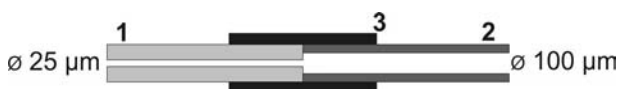
Figure 2. Detail of connection of the two capillaries: analytical capillary (1), auxiliary capillary (2) and PTFE tube (3).
