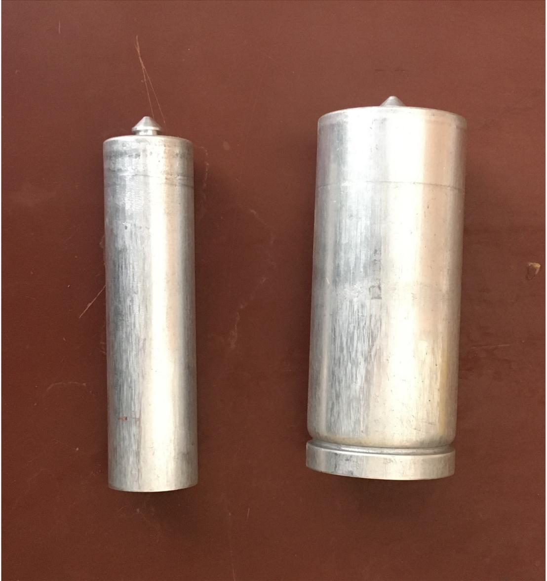
Figure 7.1: Irradiation capsules used in the experiment (larger in H6 pos., smaller in H5 pos.)
