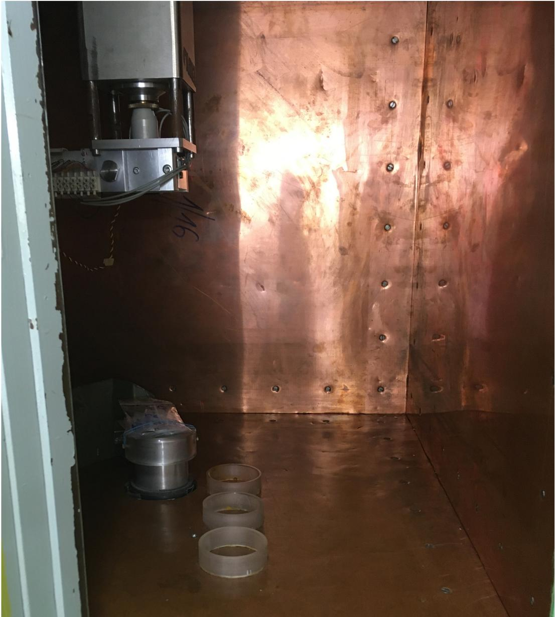
Figure 6.3: High purity Ge-crystal detector inside the shielding box with a sample handler
