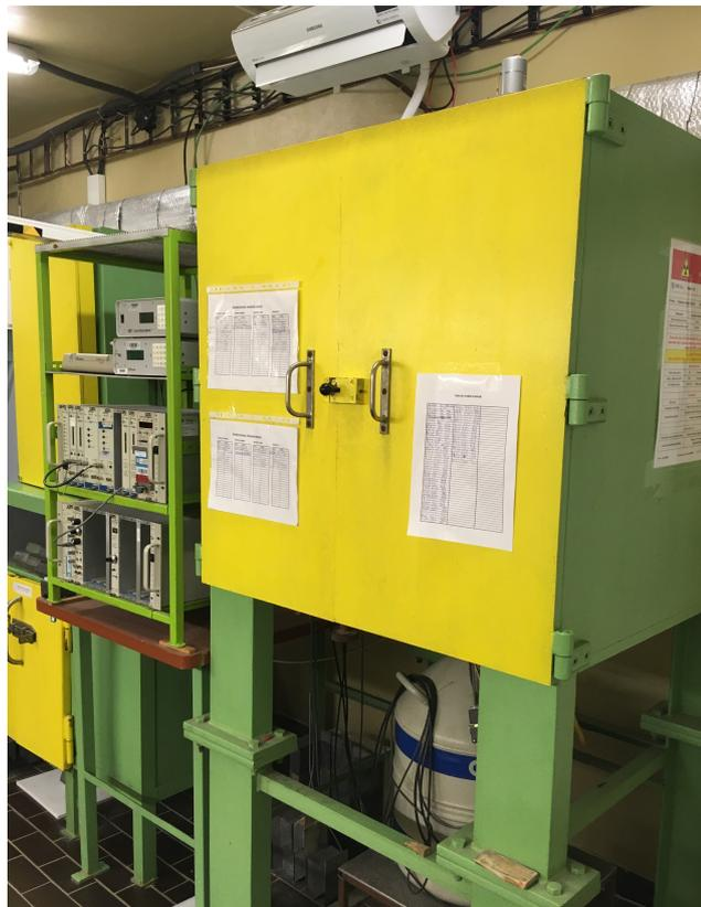
Figure 6.2:  $\gamma$ -spectrometer set up with electronics, shielding box and liquid nitrogen tank
