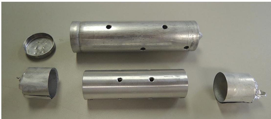
Figure 3.2: Drilled irradiation cask (upper) with a special purpose sample holder (lower)[10]
