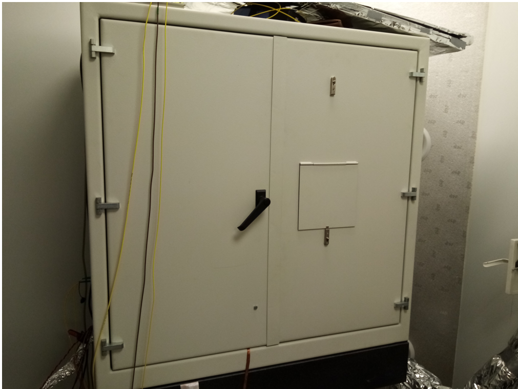
Figure 4.3: Black box used in the measurement to prevent the access of light from the room which would cause high noise.
