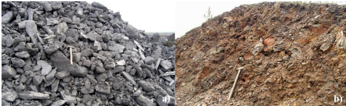
Fig. 2.3 Clay fill during the filling a) and clay fill 10 – 15 years old b) (Najser, 2010).
