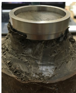
Fig. 7.1 Preparation of undisturbed sample 60386 from drill core.
