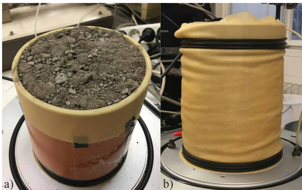
Fig. 5.4 Model 2 preparation. (a) Sample poured into the brown form. (b) Sample ready for testing.
