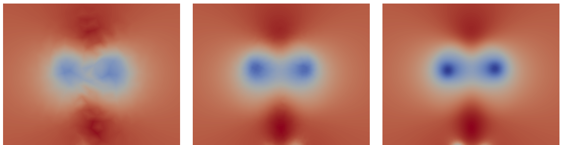
Figure 2.5: Computed pressures( u_0 = 10mm/s ) at time t=3s for different resolution of the 2D mesh (again from left 200k,600k,1.3M dof).
