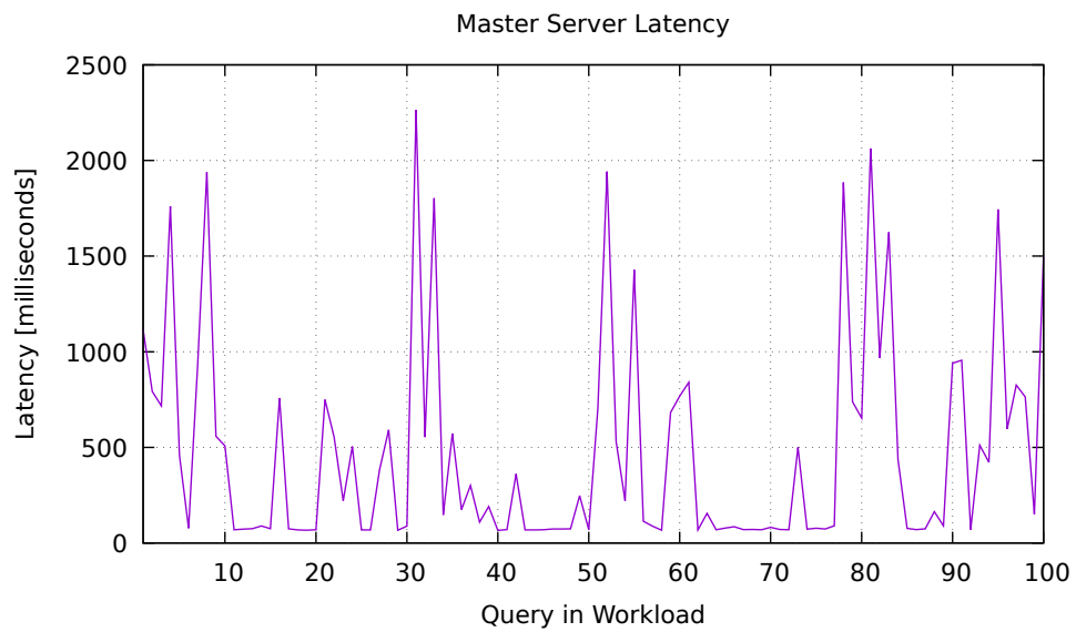
Figure 8.7: Master server latency in the Single Query workload on the Random balancing technique
