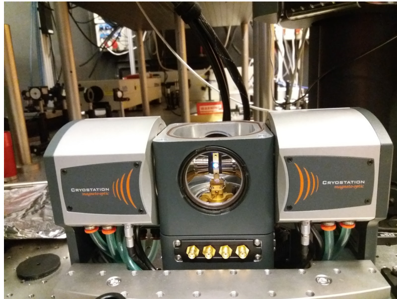
Figure 4.1: Cryostation with a sample. The field is applied IP, detection is done OOP.
