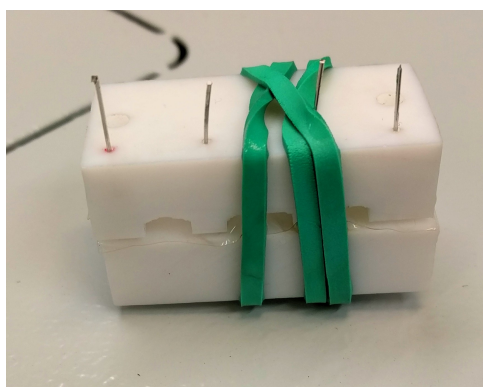
Figure 3.5: Our prototype of a screw design sample holder.
