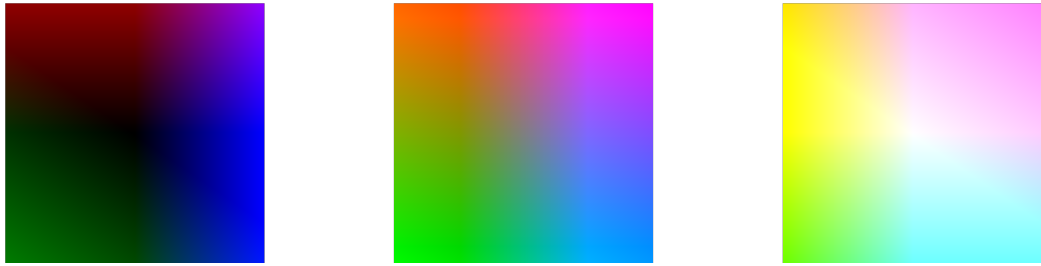
Figure 2.1: UV plane with a fixed Y value of 0, 0.5 and 1 respectively. U goes from -0.5 on the left to +0.5 on the right and V from -0.5 at the bottom to +0.5 at the top.
