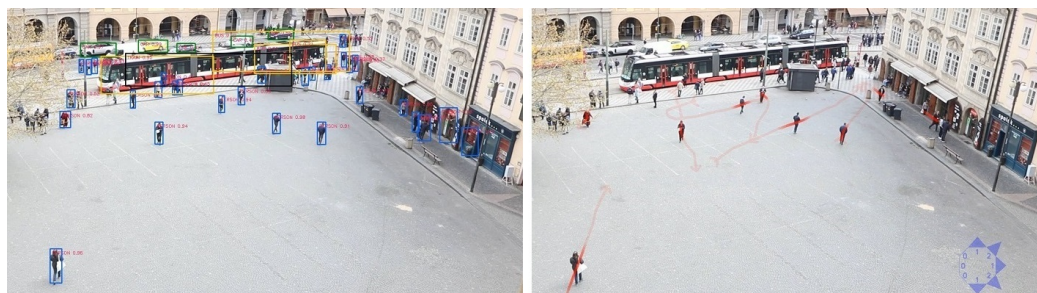
Figure 1.2: We extract basic low-level features from the video stream and further aggregate them into ones with a higher level of abstraction. Basic detections from the left image are being aggregated into trajectories of moving objects in the right image.
