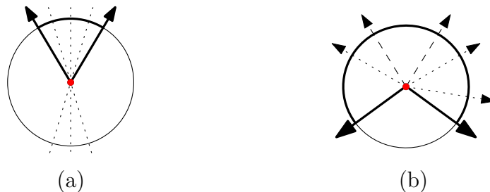
Figure 3.1: (a) Directional camera. Scene points are represented by straight lines. (b) Omnidirectional camera. Scene points are represented by half-lines. (Adopted from [6])
